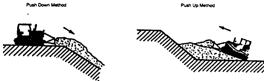
Figure 4.3 : Spreading/compaction by Push Down and Push Up method.
