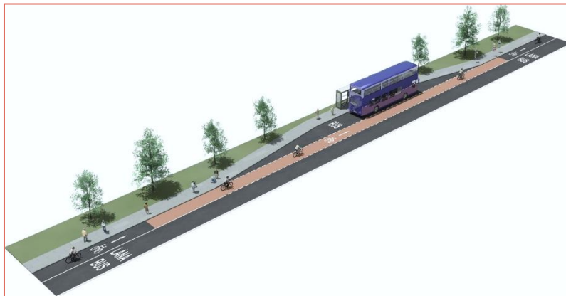
Figure 3-4: Sample picture of Bus-bay
